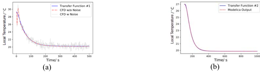
Figure 5. Comparisons between the outputs of the identified transfer functions and CFD results (a), Modelica results (b)
