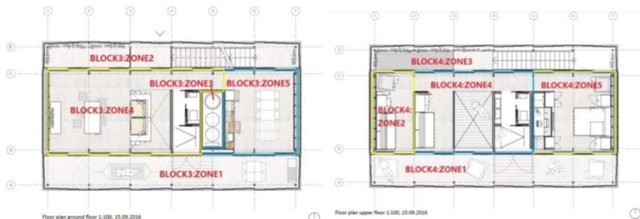
Fig. 2. Zoning in building geometric model, F1 (left), and F2 (right).
